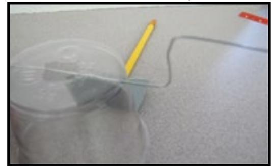
7. Bend one end into a crank.
